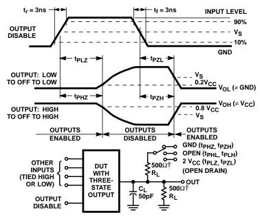
$\dagger \text{FOR}$  ac series only: when  $\text{V}_{\text{CC}}$  = 1.5V,  $\text{R}_{\text{L}}$  = 1k $\Omega$
