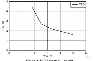
Figure 2. TPD Across V<sub>CC</sub> at 25°C
