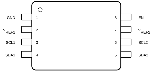
图 5-2. DCU Package 8-Pin VSSOP Top View
