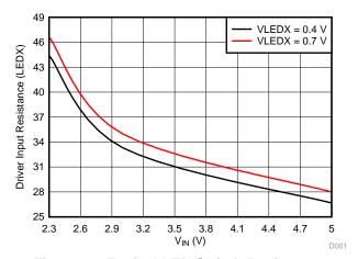
Figure 12. Typical LED Switch Resistance
