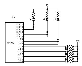
Figure 14. LP3943 Driving RGB LED as a Flash
