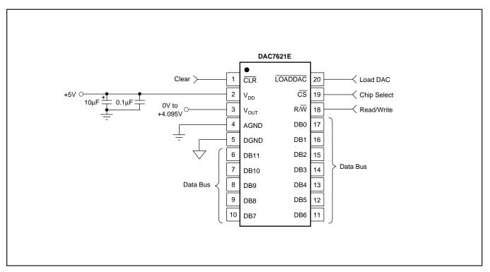
FIGURE 1. Basic Operation of the DAC7621.
