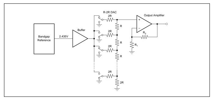
FIGURE 2. Simplified Schematic of Analog Portion.
