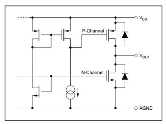
FIGURE 3. Simplified Driver Section of Output Amplifier.
