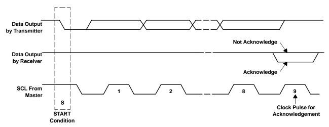
Figure 31. Acknowledge on the I<sup>2</sup>C Bus
