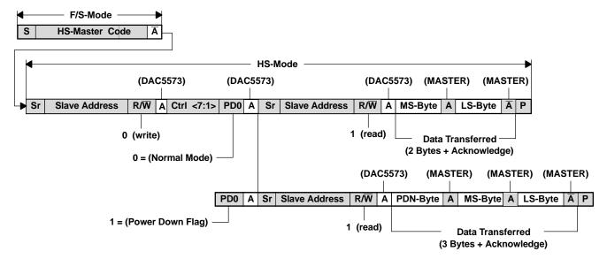
Figure 36. High-Speed Mode: Slave Transmitter
