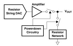
Figure 37. Output Stage During Power Down
