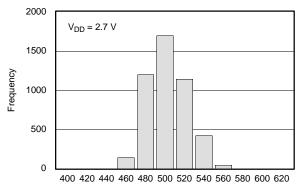
$I_{\mbox{\scriptsize DD}}$  - Current Consumption -  $\mbox{\scriptsize $\mu$A}$
