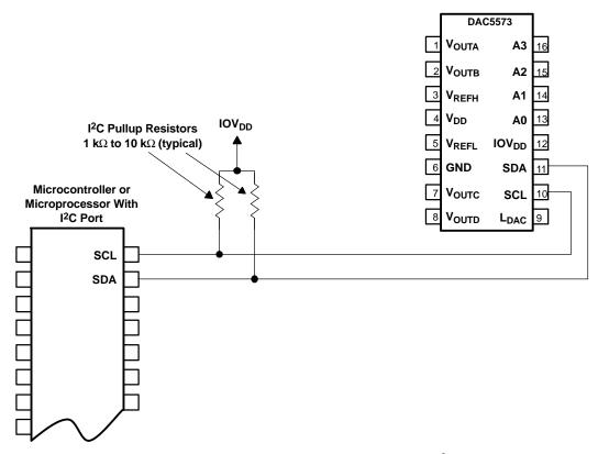
NOTE: DAC5573 power and input/output connections are omitted for clarity, except I<sup>2</sup>C Inputs.
