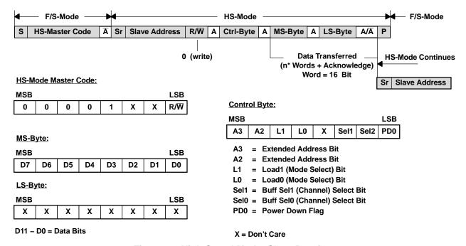
Figure 34. High-Speed Mode: Slave Receiver
