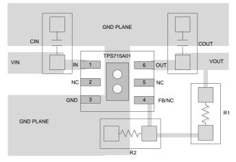
Figure 21. Example Layout for the TPS715A01DRV
