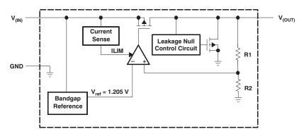
Figure 15. Functional Block Diagram—Fixed Version
