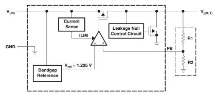
Figure 14. Functional Block Diagram—Adjustable Version
