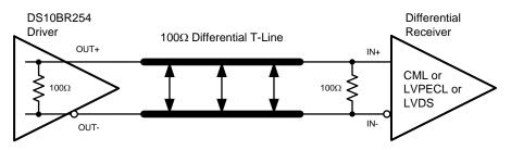
Figure 5. Typical DS10BR254 Output DC-Coupled Interface to an LVDS, CML or LVPECL Receiver
