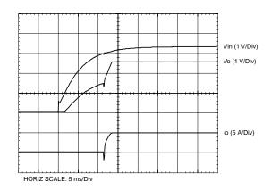
Figure 3-9; Application Circuit Demonstrating Pre-Bias Startup
