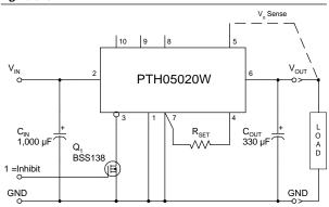
Turning  $Q_1$  on applies a low voltage to the *Inhibit* control and disables the output of the module. If  $Q_1$  is then turned off, the module will execute a soft-start power-up. A regulated output voltage is produced within 20 msec. Figure 3-4 shows the typical rise in both the output voltage and input current, following the turn-off of  $Q_1$ . The turn off of  $Q_1$  corresponds to the rise in the waveform,  $Q_1 V_{ds}$ . The waveforms were measured with a 5-A load.
