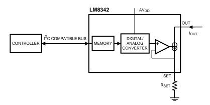
Figure 24. Block Diagram of the LM8342
