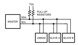
Figure 25. System Using an I<sup>2</sup>C compatible Bus
