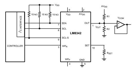
Figure 28. Typical Application Driving a V<sub>COM</sub> Level
