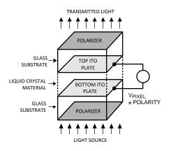
Figure 21. Individual LCD Pixel
