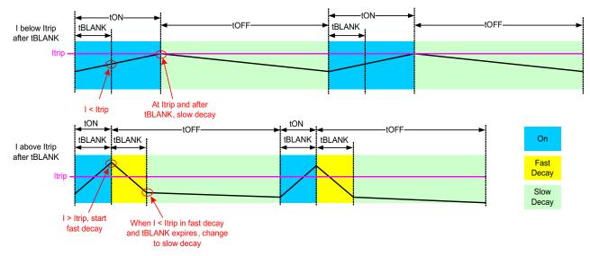
Figure 10. I < Itrip at the End of tBLANK
