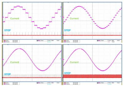
Figure 16. Microstepping Drive Current
