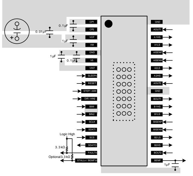
Figure 24. Recommended Layout Example
