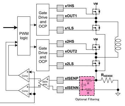
Figure 12. Optional Filtering Between R<sub>ISENSE</sub> and xINSENx
