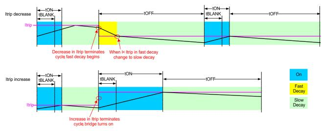
Figure 11. Itrip Level Changing During a PWM Cycle
