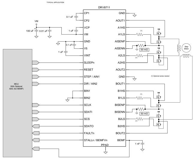
Figure 20. Typical Application Schematic
