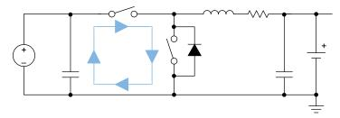
图 29. High Frequency Current Path
