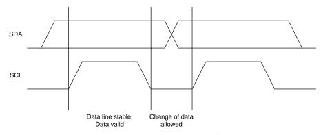
Figure 11. Bit Transfer on the I<sup>2</sup>C Bus
