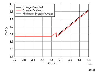
图 10. System Voltage vs Battery Voltage
