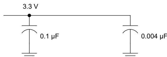
图 17. Recommended M-LVDS Bypass Capacitor Layout
