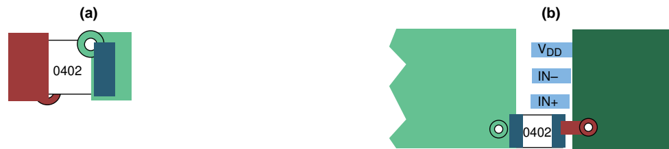
图 28. Typical Decoupling Capacitor Layouts
