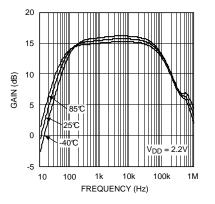
Figure 16. LMV1015-15 Gain vs. Frequency Over Temperature
