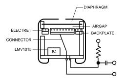
Figure 12. Built in Gain
