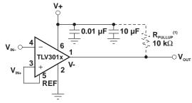
(1) Use  $R_{\text{\tiny PULLUP}}$  with the TLV3011 only.
