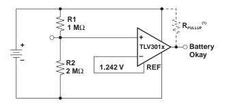
When the battery voltage drops below 1.9 V, the Battery Okay output goes low.
