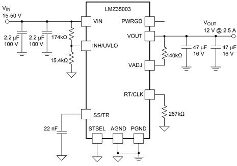
Figure 29. Typical Schematic VIN = 15 V to 50 V, VOUT = 12 V
