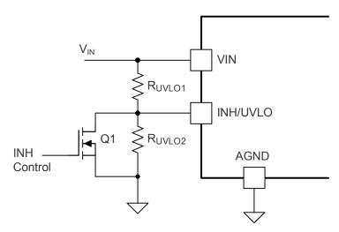
Figure 32. Typical Inhibit Control
