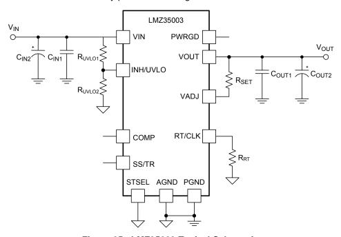
Figure 25. LMZ35003 Typical Schematic
