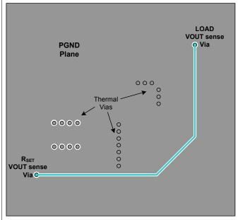
Figure 41. Typical PGND-Layer Recommended Layout
