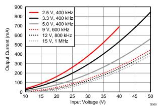
Figure 38. Pulse Skipping Threshold
