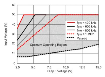
Figure 27. Optimum Operating Range with Switching Frequency
