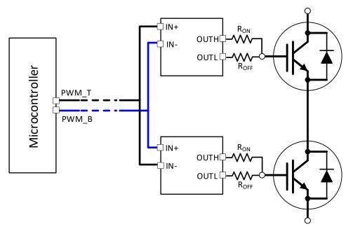
图 9-2. PWM Interlock for a Half Bridge
