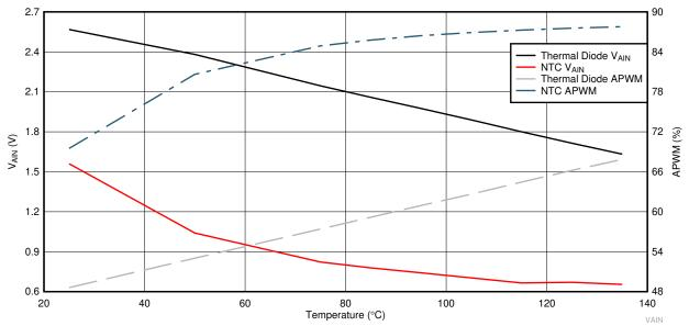
图 9-9. Thermal Diode and NTC V<sub>AIN</sub> and Corresponding Duty Cycle at APWM
