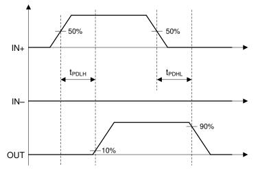
图 7-1. Non-inverting Logic Propagation Delay Measurement
