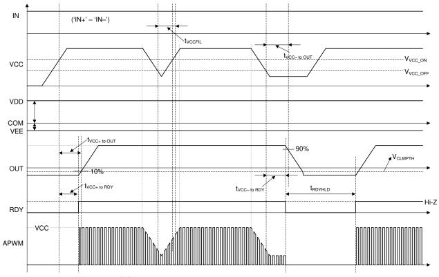
图 7-8. VCC UVLO Protection Timing Diagram
