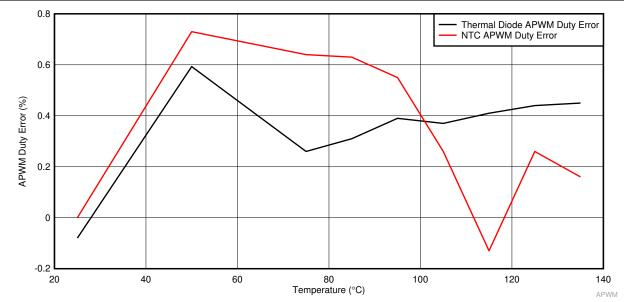
图 9-11. APWM Duty Error With Single-Point Calibration
