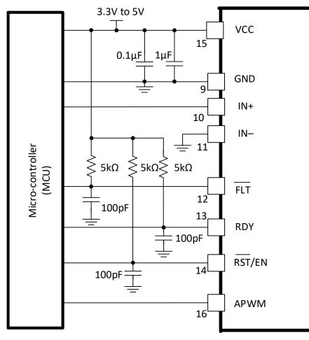
图 9-3. FLT, RDY, and RST/EN Pins Circuitry
