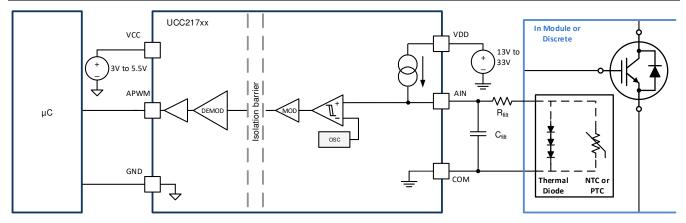
图 9-7. Thermal Diode or Thermistor Temperature Sensing Configuration
