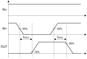
图 7-2. Inverting Logic Propagation Delay Measurement
