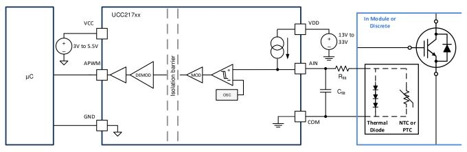
图 8-7. Isolated Analog to PWM Signal
