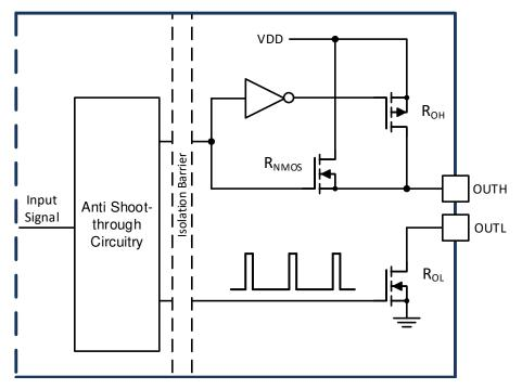
图 8-1. Gate Driver Output Stage
