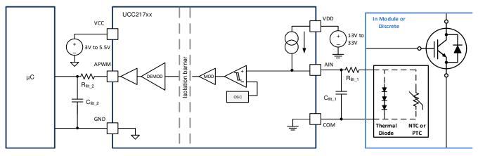
图 9-8. APWM Channel with Filtered Output
