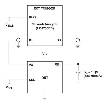
NOTE A: CL includes probe and jig capacitance.
