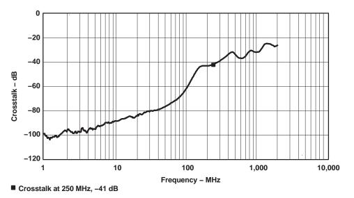
Figure 3. Crosstalk vs Frequency
