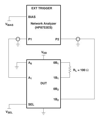
NOTES: A. C<sub>L</sub> includes probe and jig capacitance. B. A 50- $\Omega$  termination resistor is needed to match the loading of the network analyzer.
