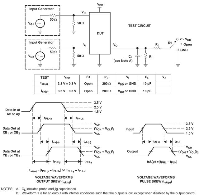
Waveform 2 is for an output with internal conditions such that the output is high, except when disabled by the output control.
