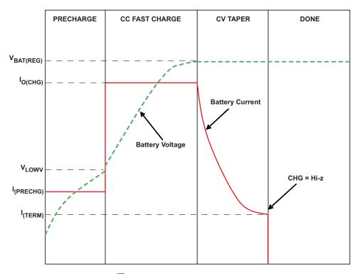
图 22. Typical Charge Cycle
