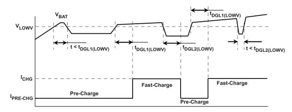
图 2. Pre- to Fast-Charge, Fast- to Pre-Charge Transition  $-t_{DGL1(LOWV)}, t_{DGL2(LOWV)}$
