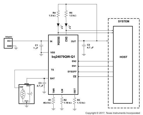
图 26. Using bq24079QW-Q1 to Disconnect the Battery from the System
