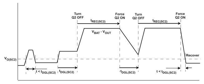
图 4. OUT Short-Circuit - Supplement Mode
