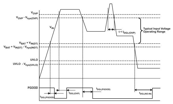
图 1. Power-Up, Power-Down, Power Good Indication
