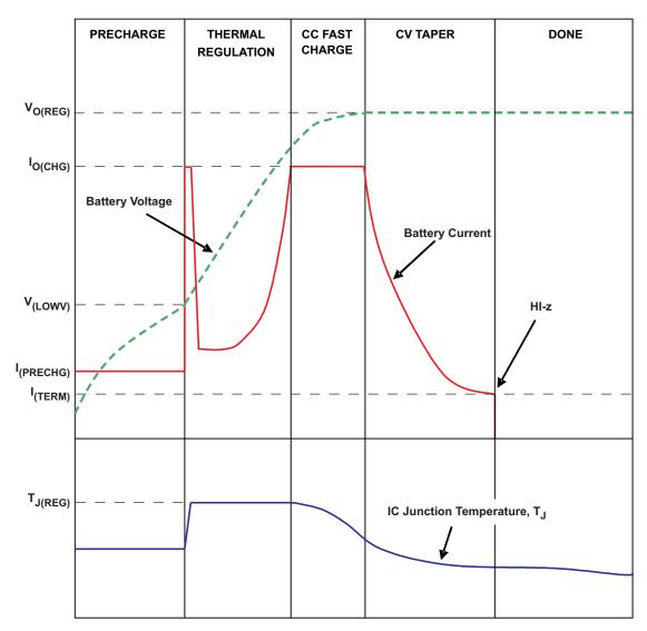
图 24. Charge Cycle Modified by Thermal Loop
