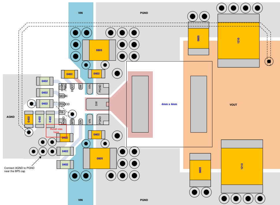
Figure 10-1. Example PCB Layout
