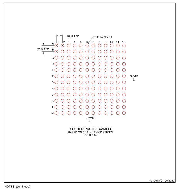
6. Laser cutting apertures with trapezoidal walls and rounded corners may offer better paste release.
