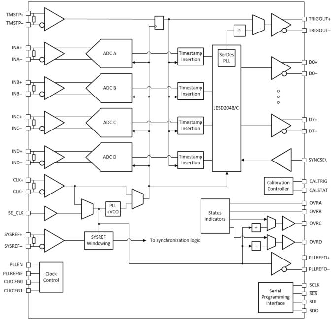
图 8-1. Quad Channel Functional Block Diagram
