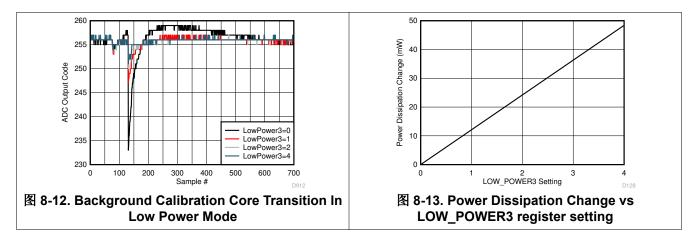
In low power background calibration mode, the timing of the ADC transition can be controlled by setting register LP\_TRIG = 1. The ADC transition will occur in the ADC output data between 500 and 1000 ADC sample clocks after triggering by the CALTRIG ball or SPI write to CAL\_SOFT\_TRIG register (Address = 0x6C).
