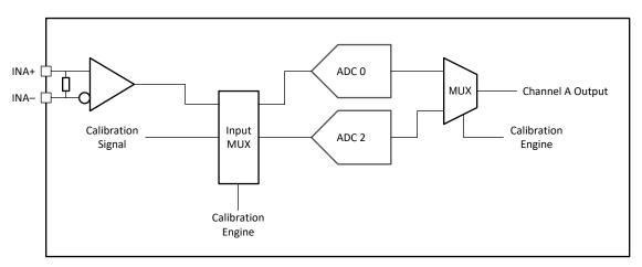
图 8-17. Single Channel Calibration System Block Diagram
