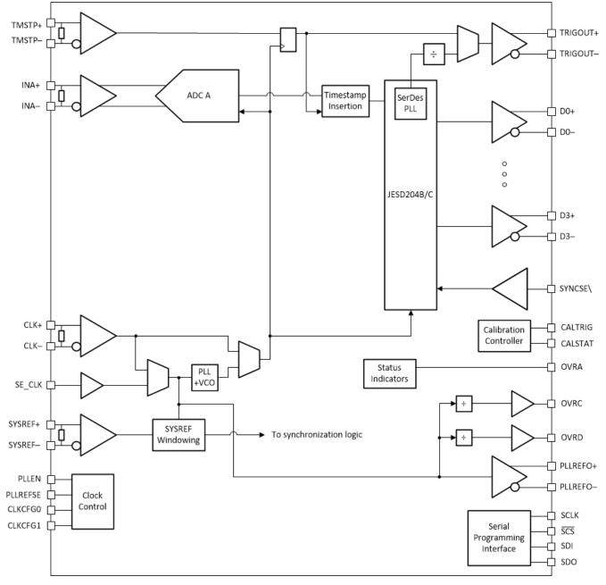
图 8-3. Single Channel Functional Block Diagram
