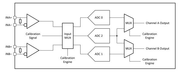
图 8-16. DualChannel Calibration System Block Diagram
