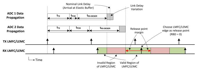
图 8-11. LMFC/LEMC Valid Region Definition for Elastic Buffer Release Point Selection
