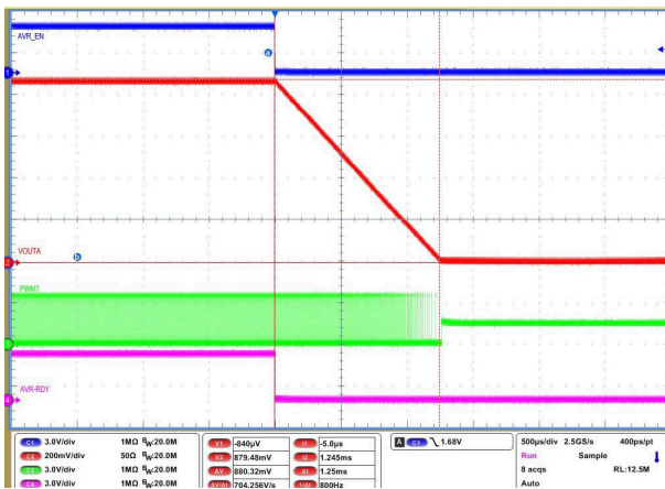
图 8-9. Soft-stop channel A (0 ms TOFF_DELAY)
