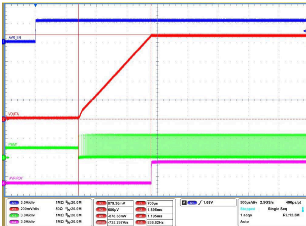
图 8-7. Soft-start channel A (0 ms TON_DELAY)
