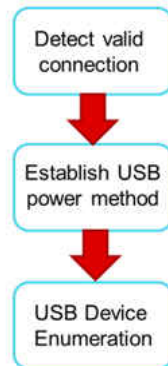
图 10-13. Flow of DFP-to-UFP Configuration
