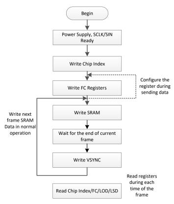
图 9-3. Design Procedure for LED Display
