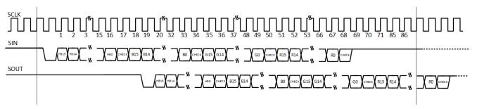
图 8-18. Data Write Command With Broadcast (Timing Diagram)
