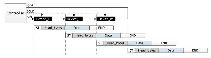
图 8-17. Data Write Command With Broadcast
