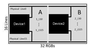
图 8-1. Two Devices in Independent Mode
