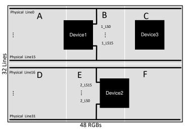
图 8-3. Three Devices in Stackable Mode
