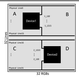
图 8-2. Two Devices in Stackable Mode
