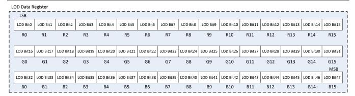
图 8-6. Bit Arrangement in LOD Data Register
