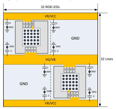
图 11-1. Power Rails Routing Suggestion
