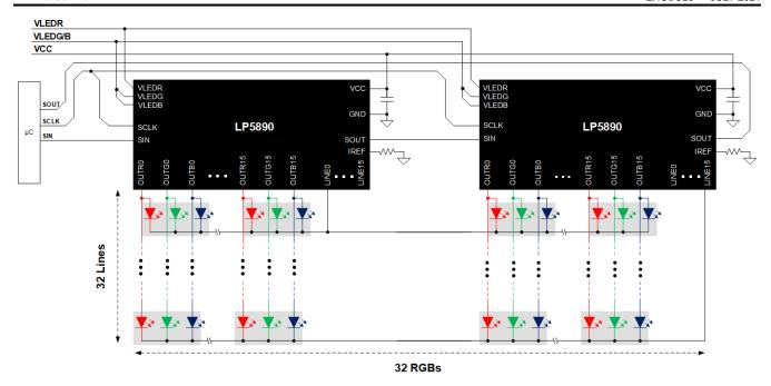
图 9-1. LP5890 with Dual Devices Stackable Connection
