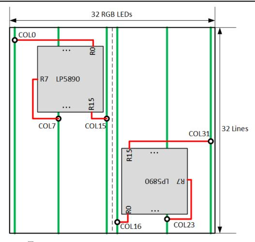
图 11-4. Channel Routing Suggestion with Channel Order Sequence
