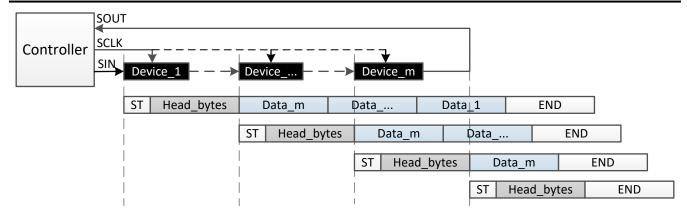
图 8-19. Data Write Command With Non-Broadcast
