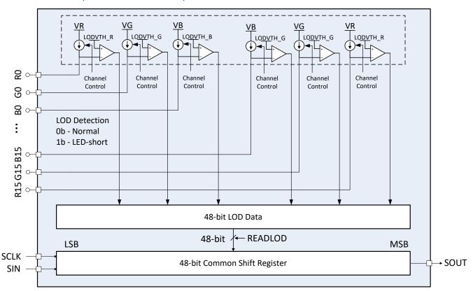
图 8-5. LED Open Detection Circuit
