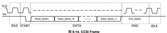
The IDLE state is not the necessary. That means the START state of next frame can connect to the END state of current frame.
