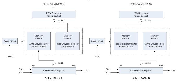
图 8-22. Bank Selection Exchange Operation
