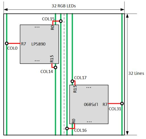
图 11-3. Channel Routing Suggestion with Shortest Wire
