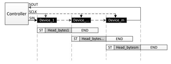
图 8-15. Chip Index Write Command
