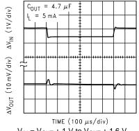
$V_{IN} = V_{OUT} + 1 V \text{ to } V_{OUT} + 1.6 V$
