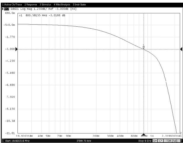
图 8-29. Data Transmission Characteristics vs Frequency (TPS25830A-Q1)
