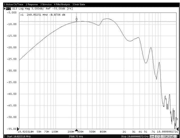
图 8-30. Off-State Data-Switch Isolation vs Frequency (TPS25830A-Q1)
