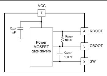
图 8-4. Internal BOOT Resistor
