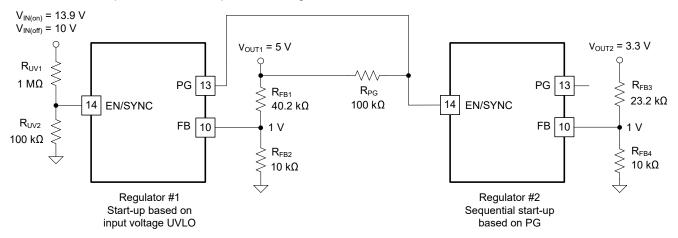
图 8-3. TPSM63604 Sequencing Implementation Using PG and EN/SYNC
