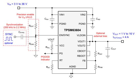
图 8-1. TPSM63604 Schematic Diagram with Input Voltage Operating Range of 3 V to 36 V
