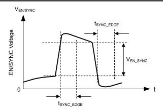
图 8-2. Typical SYNC Waveform
