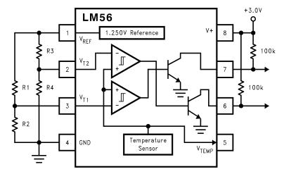
Figure 17. Reducing Errors Caused by Bias Current
