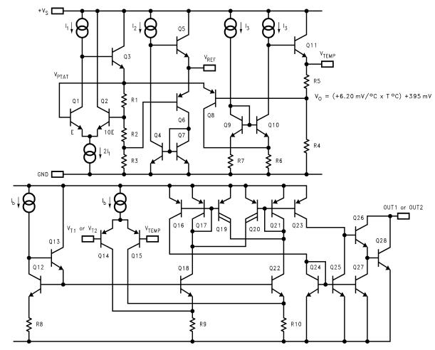
Figure 15. Simplified Schematic
