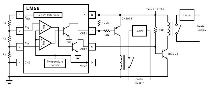
Figure 19. Simple Thermostat
