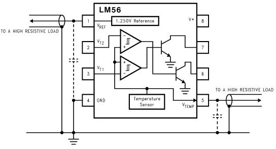
Figure 16. Loading of V<sub>REF</sub> and V<sub>TEMP</sub>
