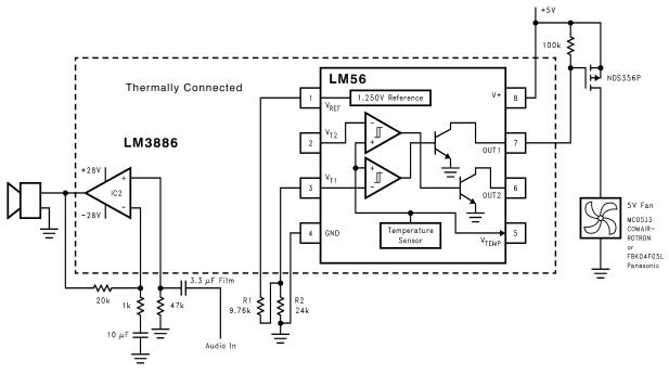
Figure 18. Audio Power Amplifier Overtemperature Detector
