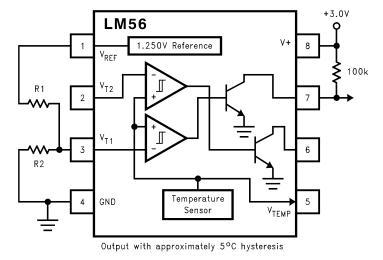
Figure 14. Single Output Configuration
