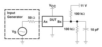
Figure 1. Device Test Setup
