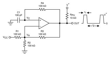
Figure 8-9. Square-Wave Oscillator
