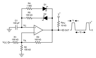
Figure 8-12. Adjustable Pulse Width Generator
