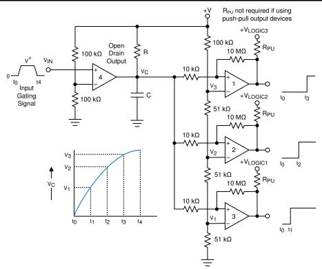
Figure 8-13. Time Delay Generator
