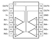
Figure 5-3. D, PW, DYY Package 14-Pin SOIC, TSSOP, SOT-23 Top View
