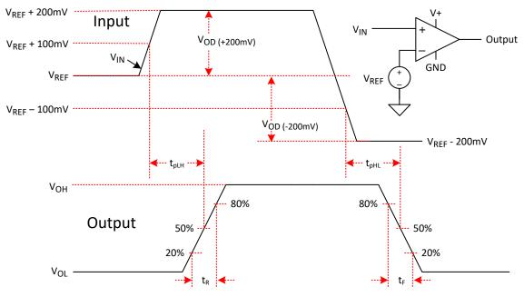
Figure 8-1. Comparator Timing Diagram
