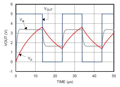
Figure 8-11. Square-Wave Oscillator Output Waveform
