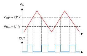
Figure 8-8. Window Comparator Results
