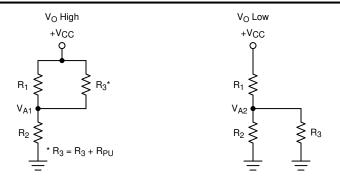
Figure 8-4. Inverting Configuration Resistor Equivalent Networks
