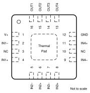
NOTE: Connect exposed thermal pad directly to GND pin.
