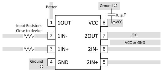
Figure 10-1. Dual Layout Example
