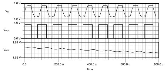
Figure 8-19. Pulse Slicer Waveforms
