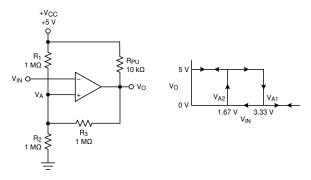
Figure 8-3. Inverting Configuration With Hysteresis
