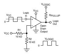
Figure 8-14. Universal Logic Level Shifter
