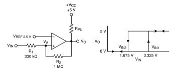
Figure 8-5. Non-Inverting Configuration With Hysteresis
