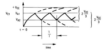
Figure 8-10. Square-Wave Oscillator Timing Thresholds
