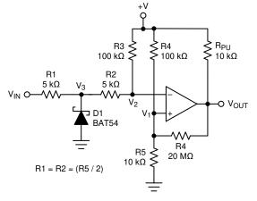
Figure 8-17. Zero Crossing Detector
