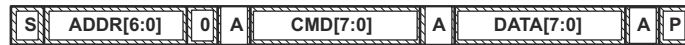
图 7-2. Attempt To Write a Read-Only Address (Nack After Data Sent By Master)
