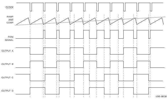
Figure 11. UCC2895-EP Timing (No Output Delay Shown)
