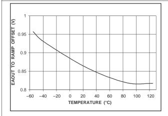
Figure 5. EAOUT To Ramp Offset Over Temperature
