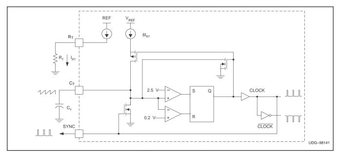
Figure 13. Oscillator Block Diagram
