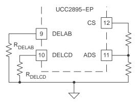
Figure 9. Resistors Needed In Programming
