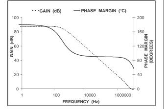
Figure 4. Error Amplifier Gain and Phase Margin
