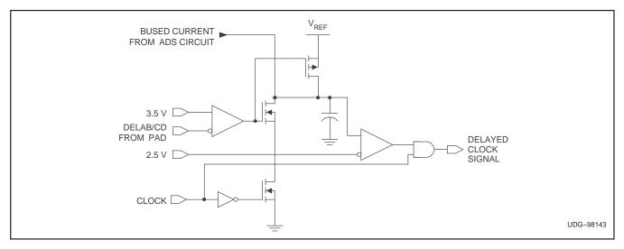
Figure 15. Delay Block Diagram (One Delay Block Per Output)
