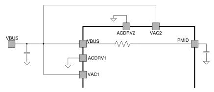
图 8-1. Single Input Connected to VBUS Directly Without ACFET-RBFET
