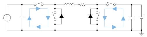
图 11-1. Buck-Boost Converter High Frequency Current Path
