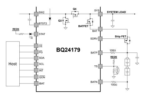
图 8-12. The Application Diagram for the External Ship FET
