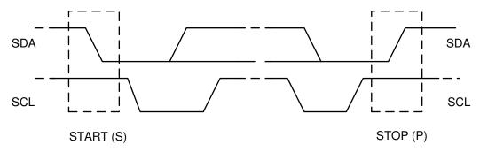
图 8-14. START and STOP Conditions on the I<sup>2</sup>C Bus
