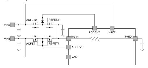
图 8-3. Two ACFETs-RBFETs Structure Supporting One Input at VAC1 and One Input at VAC2
