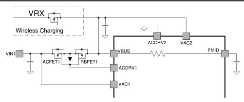
图 8-2. One ACFET-RBFET Structure Supporting One Input at VAC1 and/or One Input at VBUS
