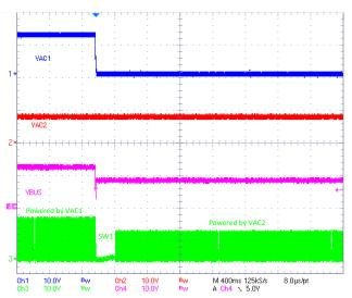
图 8-4. Input Source Auto Transition from VAC1 to VAC2 when VAC1 is Gone
