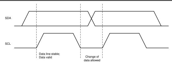
图 8-13. Bit Transfers on the I<sup>2</sup>C Bus
