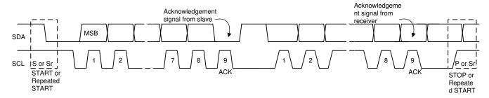
图 8-15. Data Transfer on the I<sup>2</sup>C Bus
