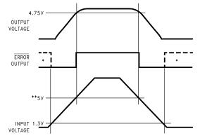
\*In shutdown mode, ERROR will go high if it has been pulled up to an external supply. To avoid this invalid response, pull-up to regulator output.
