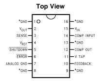
\*Internally Connected to Power Ground
