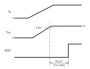
$*R_{T} = 1 \text{ Meg}, C_{T} = 0.1 \ \mu\text{F}$
