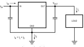
$P_{D} = (V_{IN} - V_{OUT}) |_{L} + (V_{IN}) |_{G}$
