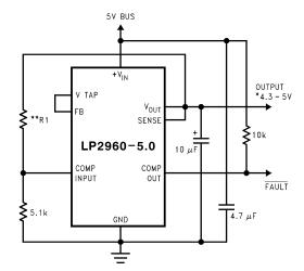
\*Output voltage equals +V<sub>IN</sub> minus dropout voltage, which varies with output current. Current limits at a maximum of 1000 mA (typical).
