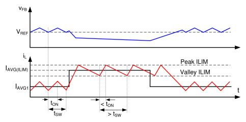
图 11. Current Limit Timing Diagram
