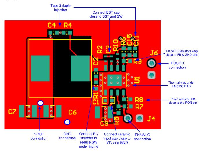
图 30. LM5163 Single-Sided PCB Layout Example
