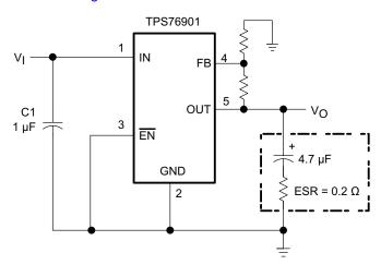
Figure 5. Typical Application Circuit
