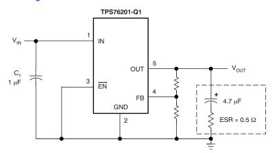
Figure 18. Typical Application Circuit
