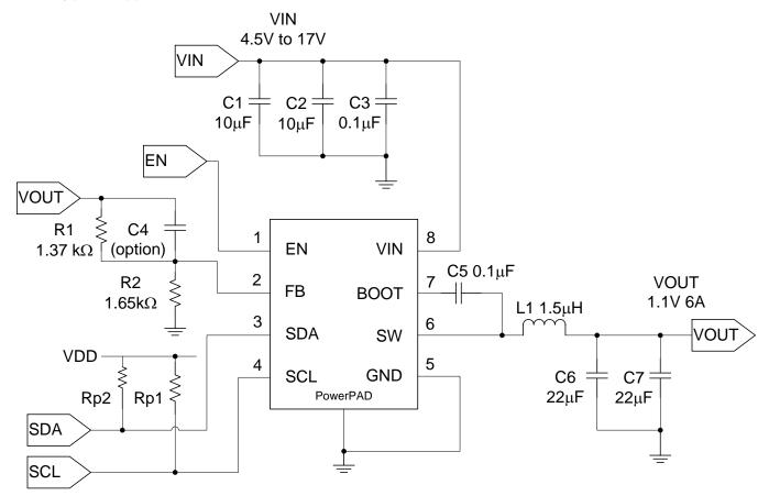
Figure 17. Typical Application Schematic
