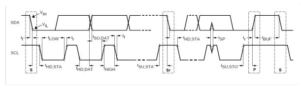
Figure 1. I<sup>2</sup>C Timing Definitions (reproduced from Phillips I<sup>2</sup>C spec Version 1.1)
