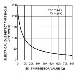
Figure 7. Typical Idle Threshold vs. SD\_TH resistor value
