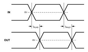
Figure 4. Propagation Delay Timing Diagram
