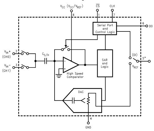
\*For ADC08831  $V_{REF}$  pin is available, for ADC08832 DI pin is available, and  $V_{REF}$  is tied to  $V_{CC}$  Pin names in parentheses refer to ADC08832
