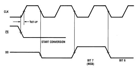
Figure 19. ADC08831 Start Conversion Timing
