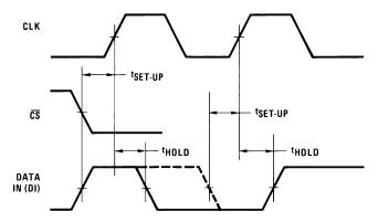
Figure 17. Data Input Timing
