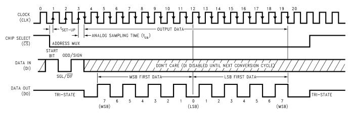
Figure 21. ADC08832 Timing
