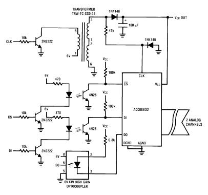
Figure 29. Isolated Data Converter
