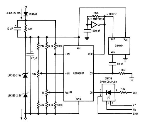
All power supplied by loop 1500V isolation at output
