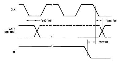
Figure 18. Data Output Timing
