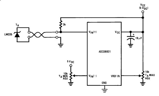
Figure 23. Low-Cost Remote Temperature Sensor
