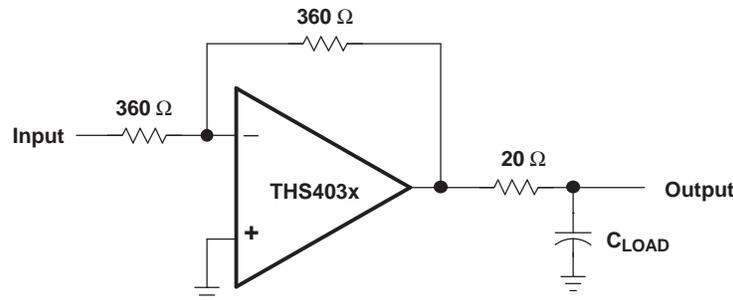
图 53. Driving a Capacitive Load
