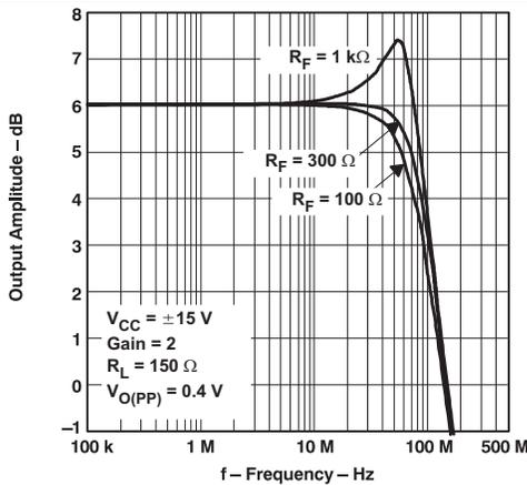
图 29. Small-Signal Frequency Response With Varying Feedback Resistance
