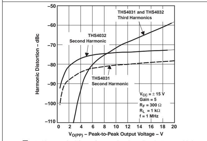
图 17. Harmonic Distortion vs Peak-to-Peak Output Voltage
