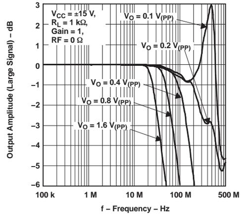
图 22. Frequency Response With Varying Output Voltage Swing
