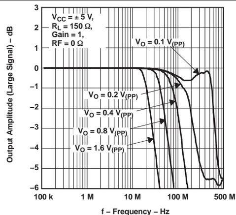
图 28. Frequency Response With Varying Output Voltage Swing
