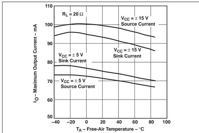
图 7. Maximum Output Current vs Free-Air Temperature
