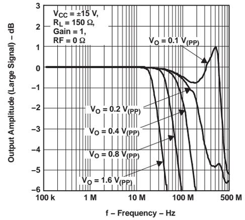
图 24. Frequency Response With Varying Output Voltage Swing
