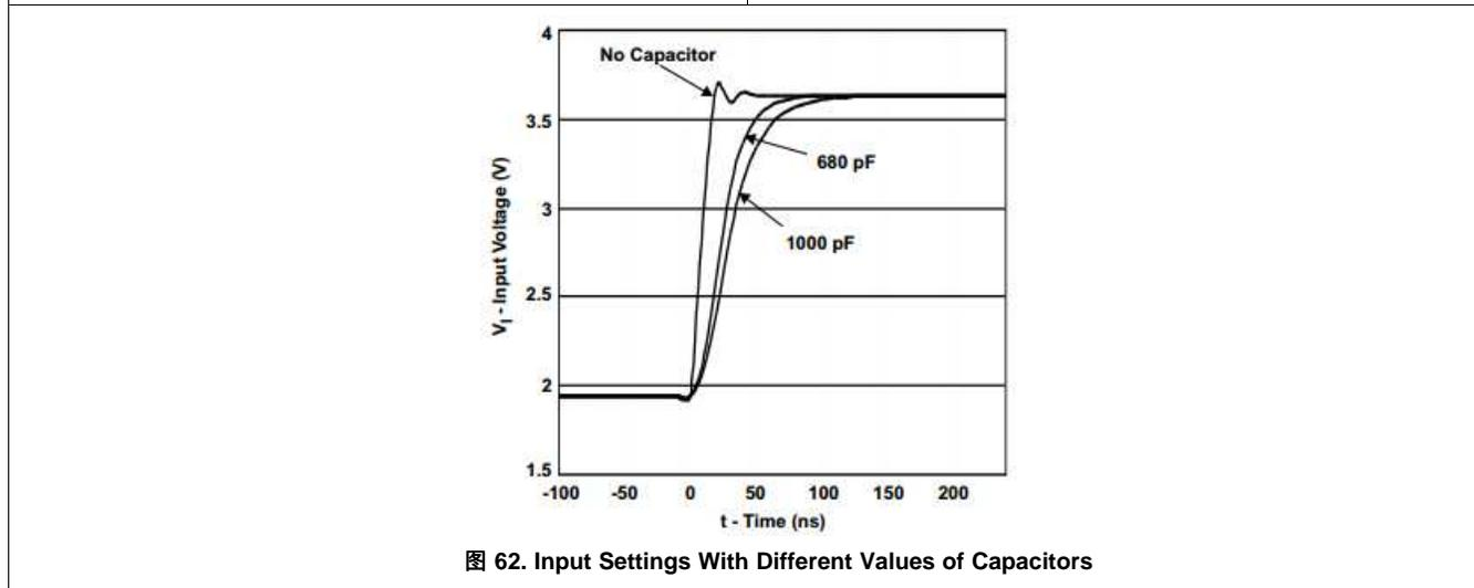
图 62. Input Settling With Different Values of Capacitors
