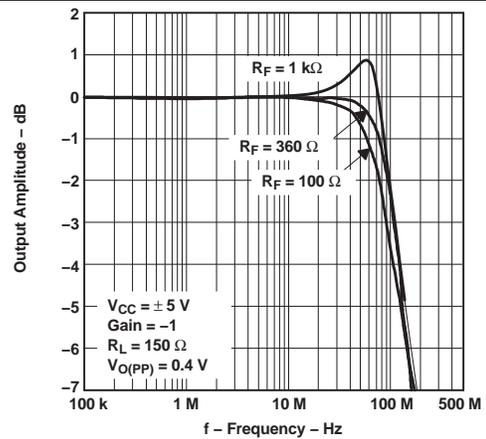
图 32. Small-Signal Frequency Response With Varying Feedback Resistance
