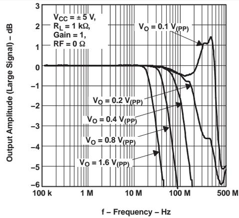
图 26. Frequency Response With Varying Output Voltage Swing
