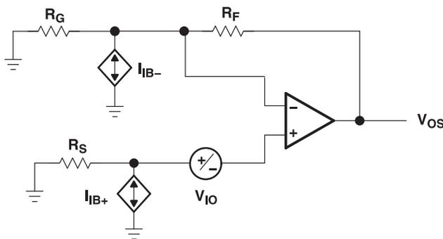
$$V_{OS} = (\pm V_{IO} \pm I_{IB+} R_S) \left( 1 + \frac{R_F}{R_G} \right) \pm I_{IB-} R_F$$
