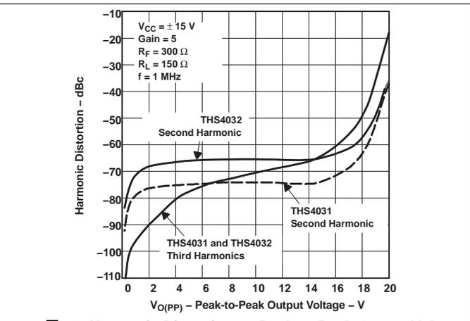
图 18. Harmonic Distortion vs Peak-to-Peak Output Voltage
