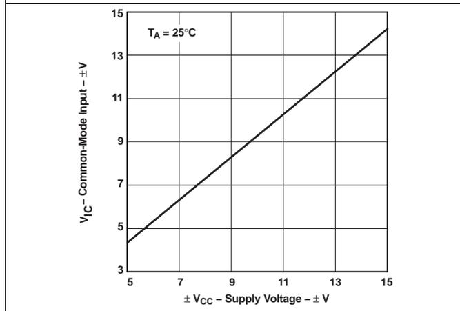
图 9. Common-Mode Input Voltage vs Supply Voltage
