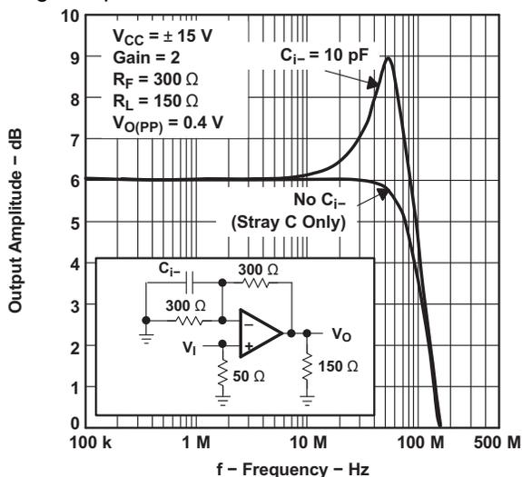
**图 51. Output Amplitude vs Frequency**
