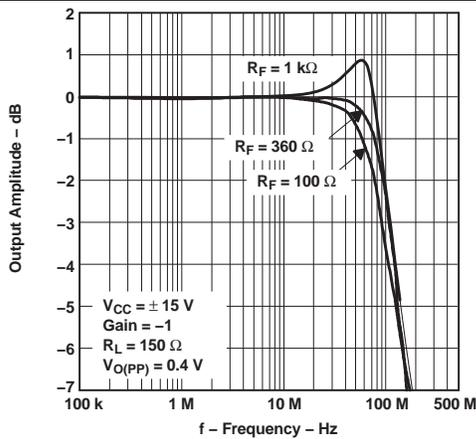
图 31. Small-Signal Frequency Response With Varying Feedback Resistance
