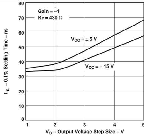
图 20. 0.1% Settling Time vs Output Voltage Step Size
