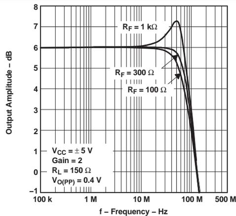
图 30. Small-Signal Frequency Response With Varying Feedback Resistance
