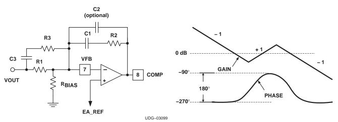
Figure 7. Type III Compensation Configuration
