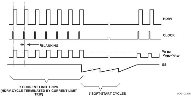
Figure 4. Typical Current Limit Protection Waveforms
