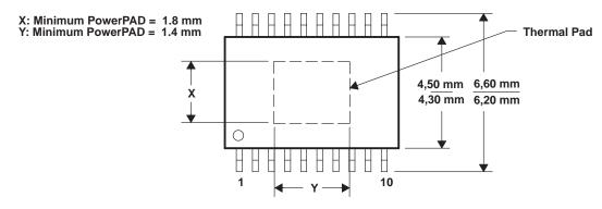
Figure 10. PowerPAD Dimensions
