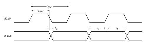
Figure 2. Modulator Output Mode Timing
