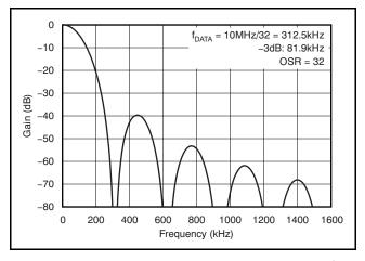
Figure 25. Frequency Response of the Sinc<sup>3</sup> Filter
