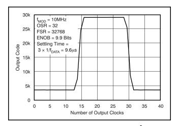
Figure 26. Pole Response of the Sinc<sup>3</sup> Filter
