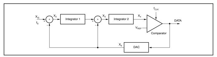
Figure 24. Block Diagram of the 2nd-Order Modulator
