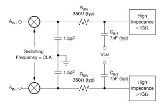
Figure 1. Equivalent Analog Input Circuit
