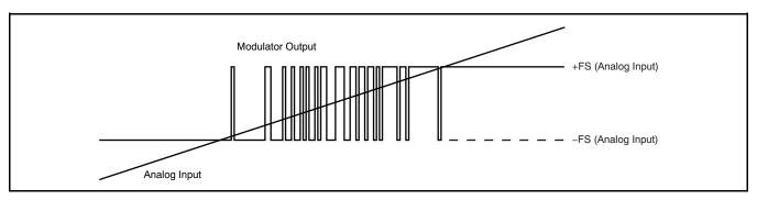
Figure 27. Analog Input vs Modulator Output
