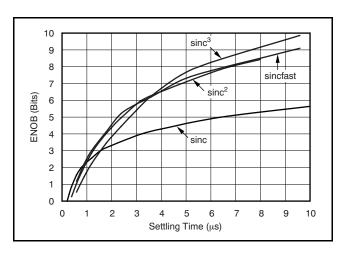
Figure 29. Measured Effective Number of Bits vs Settling Time
