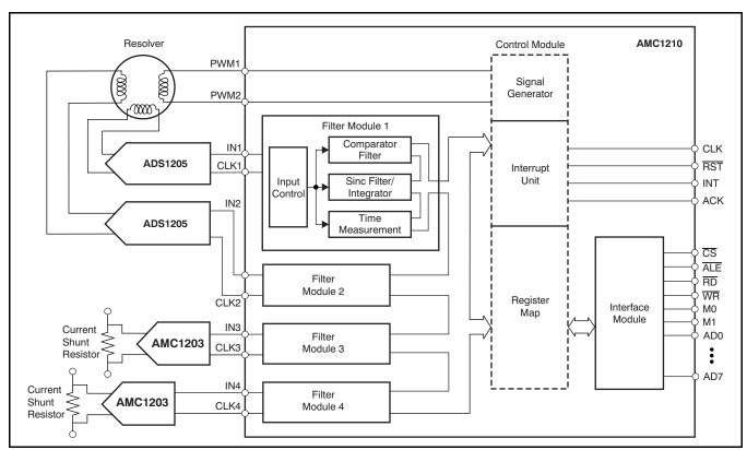
Figure 23. Example of a Resolver-Based Motor-Control Application
