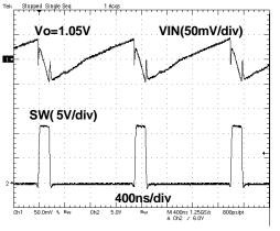
Figure 15. VOLTAGE RIPPLE AT INPUT (I<sub>O</sub> = 6 A)
