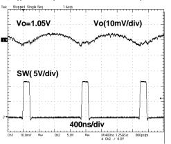
Figure 13. VOLTAGE RIPPLE AT OUTPUT (I<sub>O</sub> = 6 A)
