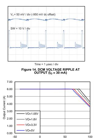
T<sub>a</sub> Ambient Temperature (°C) Figure 16. OUTPUT CURRENT vs AMBIENT TEMPERATURE
