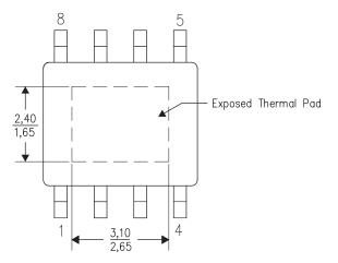
Figure 18. Thermal Pad Dimensions
