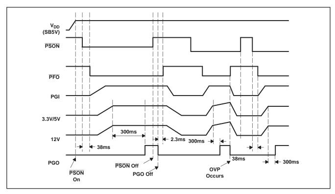
Figure 1. AC Turn-On and Over-Voltage Protect
