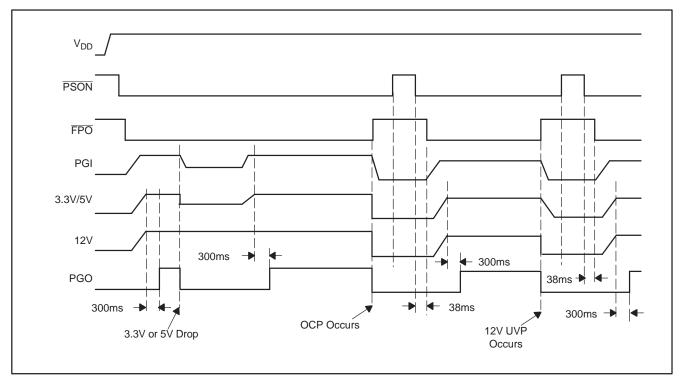
Figure 2. Over-Current and Under-Voltage Detect/Protect
