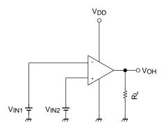
$$V_{\text{IN1}} = \frac{V_{\text{DD}}}{2} - 0.05 \text{ V}$$
