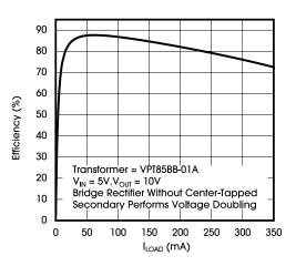
Figure 9. Efficiency vs. Load Current (5V-10V)
