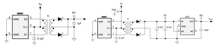
Figure 22. Unregulated Output for Low-Current Loads with Wide Supply Range
