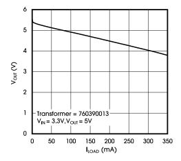
Figure 6. Output Voltage vs. Load Current (3.3V-5V)
