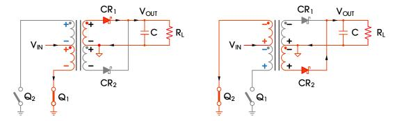
Figure 17. Switching Cycles of a Push-Pull Converter
