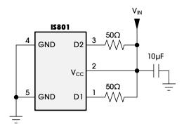
Figure 15. Test Circuit For  $R_{\text{ON}},\,F_{\text{SW}},\,F_{\text{St}},\,T_{\text{r-D}},\,T_{\text{f-D}},\,T_{\text{BBM}}$
