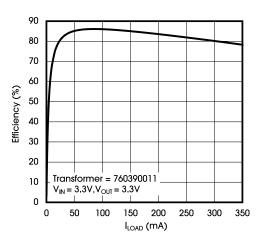
Figure 3. Efficiency vs. Load Current (3.3V-3.3V)
