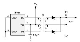
Figure 12. Measurement Circuit for Unregulated Output (TP1)
