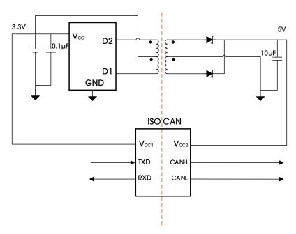
Figure 20. Typical Application Schematic (IS801)
