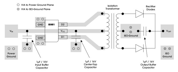
Figure 24. Layout Example of a 2-Layer Board (IS801)
