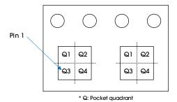
Figure 27. Product Loading Orientation
