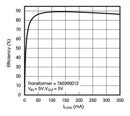
Figure 5. Efficiency vs. Load Current (5V-5V)
