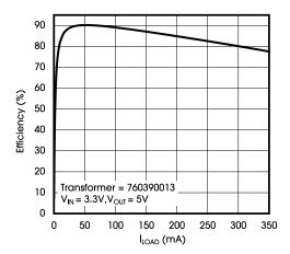
Figure 7. Efficiency vs. Load Current (3.3V-5V)
