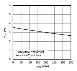
Figure 2. Output Voltage vs. Load Current (3.3V-3.3V)
