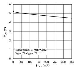
Figure 4. Output Voltage vs. Load Current (5V-5V)
