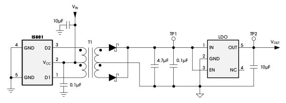
Figure 14. Measurement Circuit for Regulated Output (TP1 and TP2)
