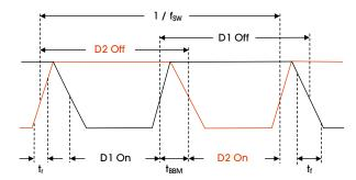
Figure 13. Timing Diagram
