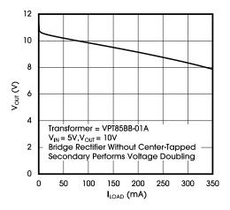
Figure 8. Output Voltage vs. Load Current (5V-10V)
