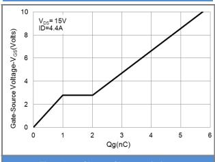
**Fig.7 Gate-Charge Characteristics**
