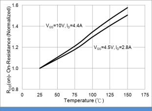
Fig.4 On-Resistance vs. Junction temperature
