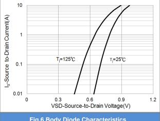
Fig.6 Body Diode Characteristics
