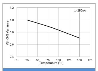
Fig.8 Threshold Voltage Variation with Temperature.
