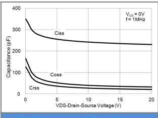
Fig.9 Capacitance vs. Drain-Source Voltage.
