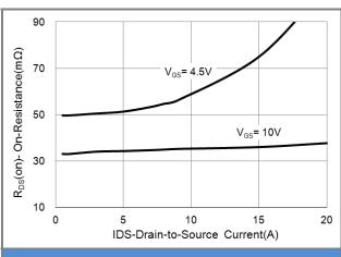
Fig.3 On-Resistance vs. Drain Current
