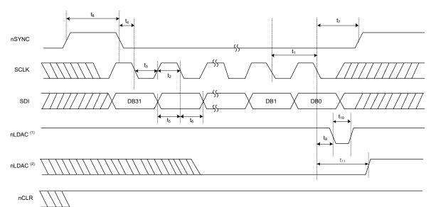
NOTES: 1. Asynchronous update mode. DAC is updated at the falling edge of nLDAC. 2. Synchronous update mode. nLDAC can be tied low permanently.
