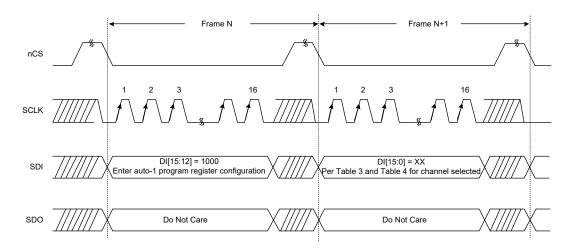
NOTE: During the programming process, the chip continues to run in the selected mode. The SDO is valid, but it is impossible to change the range or write GPIO data to the device during programming.
