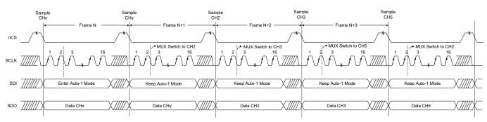
Figure 6. Example for Auto-1 Mode Timing Diagram
