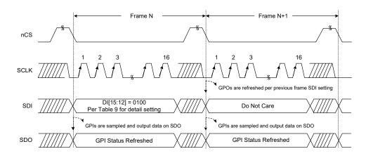
NOTE: During the programming process, the chip continues to run in the selected mode. The SDO is valid, but it is impossible to change the range or write GPIO data to the device during programming.
