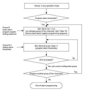
NOTE: During the programming process, the chip continues to run in the selected mode. The SDO is valid, but it is impossible to change the range or write GPIO data to the device during programming.
