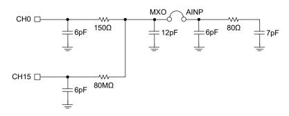
NOTE: CH0 is assumed to be on, and CH15 is assumed to be off. Figure 12. Equivalent Circuit for ADC and MUX
