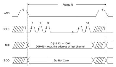
NOTE: During the programming process, the chip continues to run in the selected mode. The SDO is valid, but it is impossible to change the range or write GPIO data to the device during programming.
