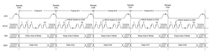
Figure 8. Example for Auto-2 Mode Timing Diagram
